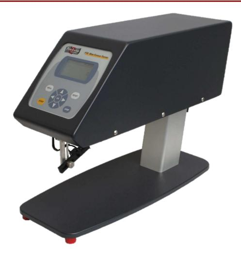
**Rotating Beam Wire Fatigue Tester Model FTX** Tests wires to failure by rotating the specimen such that it is bent through 180 degrees, causing a once-per-revolution bending stress cycle in the specimen. Unlike competitive machines, the wire is driven from both ends eliminating the possibility of induced torque in the wire.
